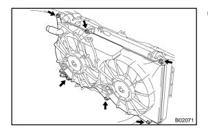
(f) Remove the 6 bolts and cooling fan.
