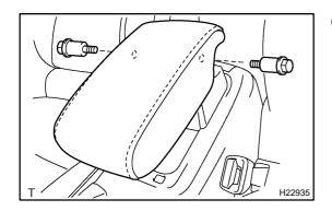
(b) Remove the 2 bolts and remove the console compartment door.
