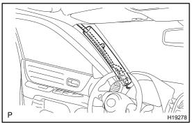
(e) Cover the airbag with protective cover as shown in the illustration...
