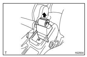
(c) Remove the console box cover rear.
