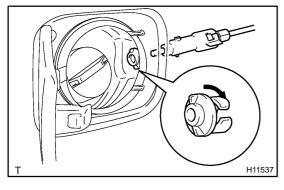
(b) Insert the fuel lid lock control to the retainer and rotate it to the left to lock.
