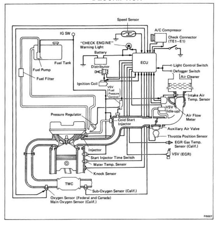
The EFI system is composed of 3 basic subsystems; Fuel, Air Induction and Electronic Control Systems.
