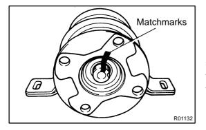
(k) Align the matchmarks on the universal joint flange and intermediate shaft, and install the universal joint flange.
