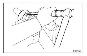
(c) Using SST and press, install a new dust cover. SST 09316-6001 1 (09316-00011)
