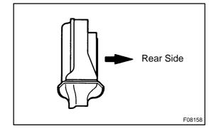
(i) Install a new center support bearing to intermediate shaft. HINT:
