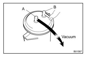
(c) Plug port B with your finger, and apply 53.3 kPa (400 mmHg, 15.75 in.Hg) of vacuum to port A, and check that there is no change in vacuum after 1 minute.
