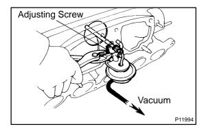
If operation is not as specified, turn the adjusting screw.
