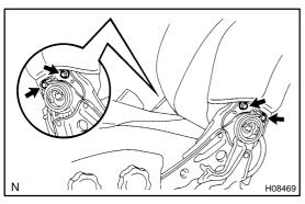
(d) Remove the 4 bolts and move the seatback assembly a little upward.
