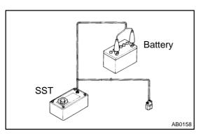
(c) Check functioning of the SST. SST 09082–00700
