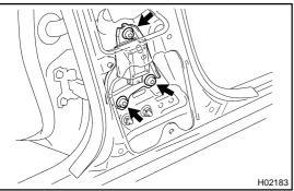
3. REMOVE SIDE AIRBAG SENSOR ASSEMBLY
