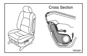
Check that there are no cuts or the frayed on seams and out side of seatback cover.
