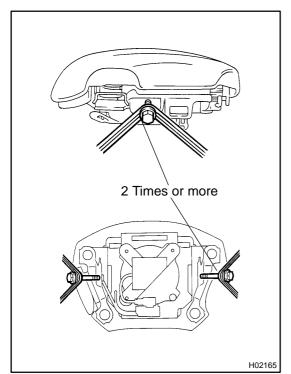
(3) Using 3 wire harnesses, wind the wire harness at least 2 times each around the bolts installed on the left and right sides of the steering wheel pad.
