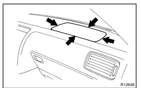
There should be no interference between the instrument panel and the front passenger airbag assembly.
