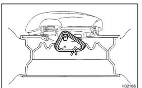
(4) Face the upper surface of the steering wheel pad upward. Separately tie the left and right sides of the steering wheel pad to the disc wheel through the hub nut holes. Position the steering wheel pad connector so that it hangs downward through a hub hole in the disc wheel.
