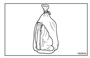
(f) Dispose of the side airbag assembly.
