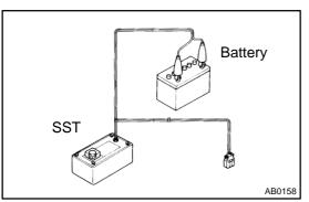
1. AIRBAG DEPLOYMENT WHEN SCRAPPING VE-HICLE
