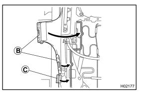
(b) Hang the hook "B" and "C" onto the seatback frame. **CAUTION:**
