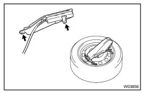
(2) Put the wire harness through the holes shown in the illustration and then tie and fix the wheel with tire.
