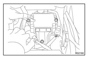
2. REMOVE AIRBAG SENSOR ASSEMBLY
