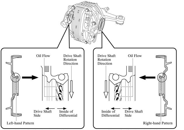
**Rear Differential Side Gear Shaft Oil Seal LH**
